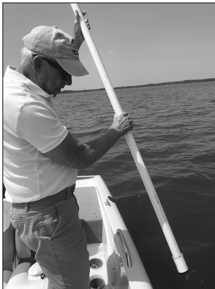
Marty Cook, LLA volunteer, uses a water sampling tube to take water from Kabekona Bay.
